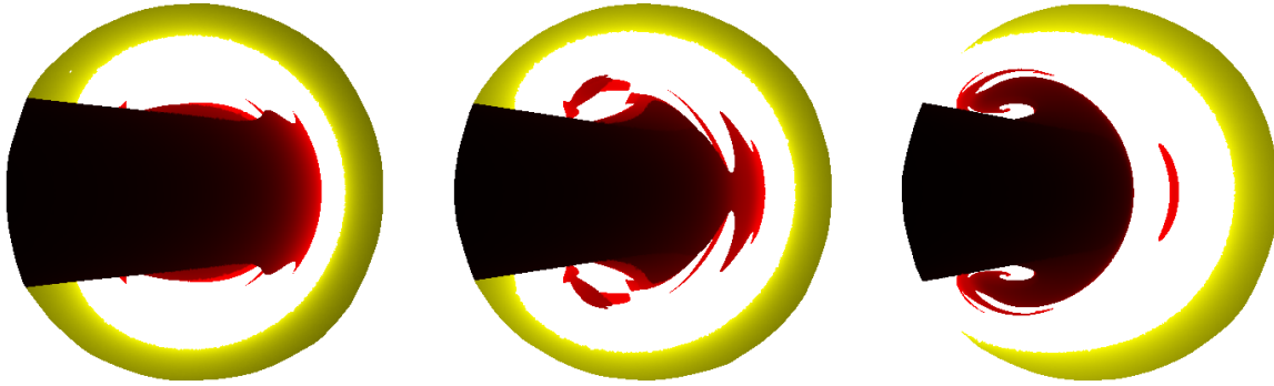
Figure 3.9: Impact and escape sets for out-of-plane maneuvers by an orbiter of a rotating ellipsoid as rotation rate, triaxiality, and third body perturbations are incremented simultaneously.
